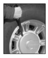
To remove the center cap, place the flat end of the wheel wrench in the slot on the wheel and gently pry the center cap out.
